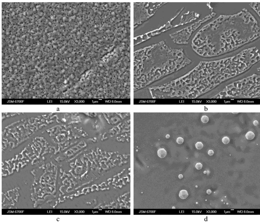
**Fig. 3.** SEM images of the titanium nanofilms on the ZrO<sub>2</sub>-ceramic after annealing in vacuum at 1600°C with different holding time: a – 2 min; b – 5 min; c – 10 min; d – 20 min.
