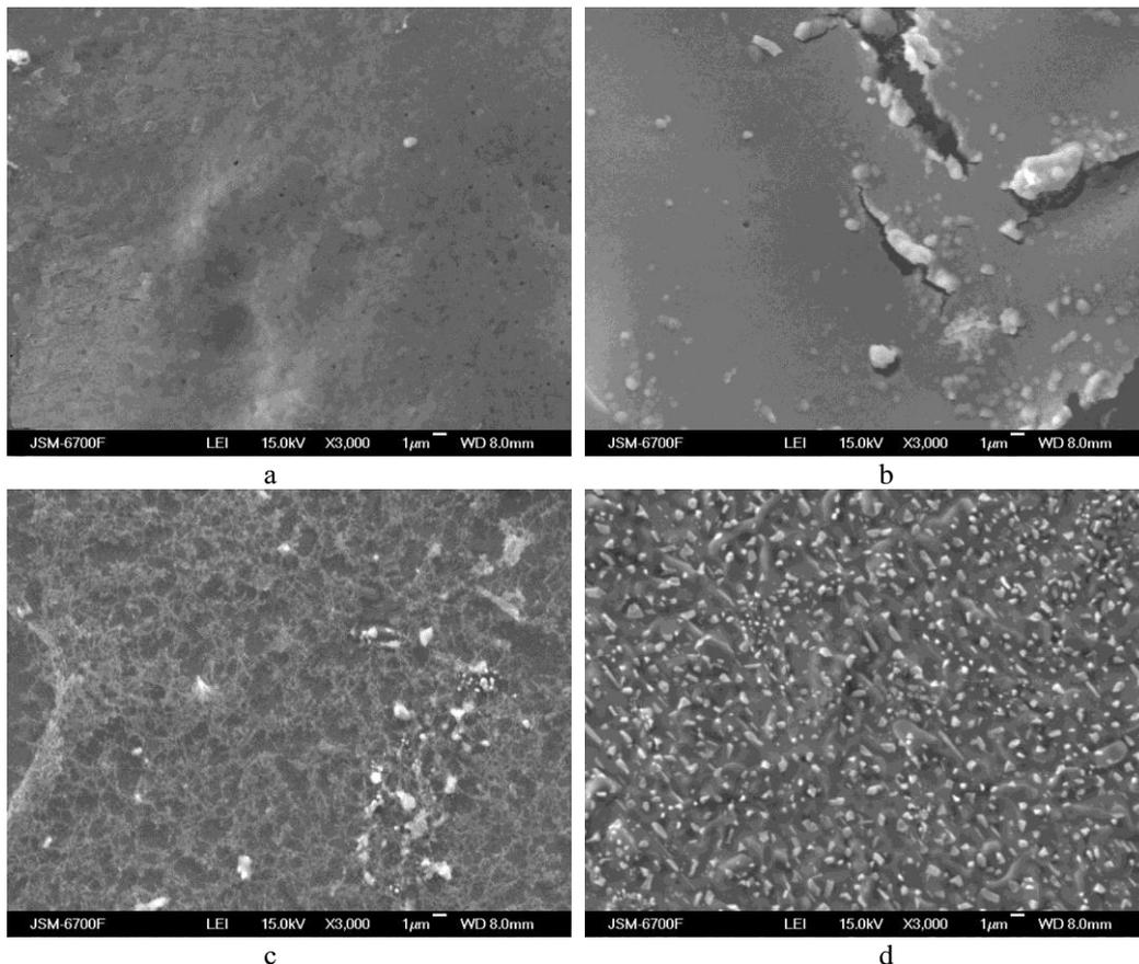
**Fig. 1.** SEM image of the titanium nanofilms onto ZrO<sub>2</sub>-ceramic after annealing in vacuum at 1400°C with different holding time: a – 2 min; b – 5 min; c – 10 min; d – 20 min.
