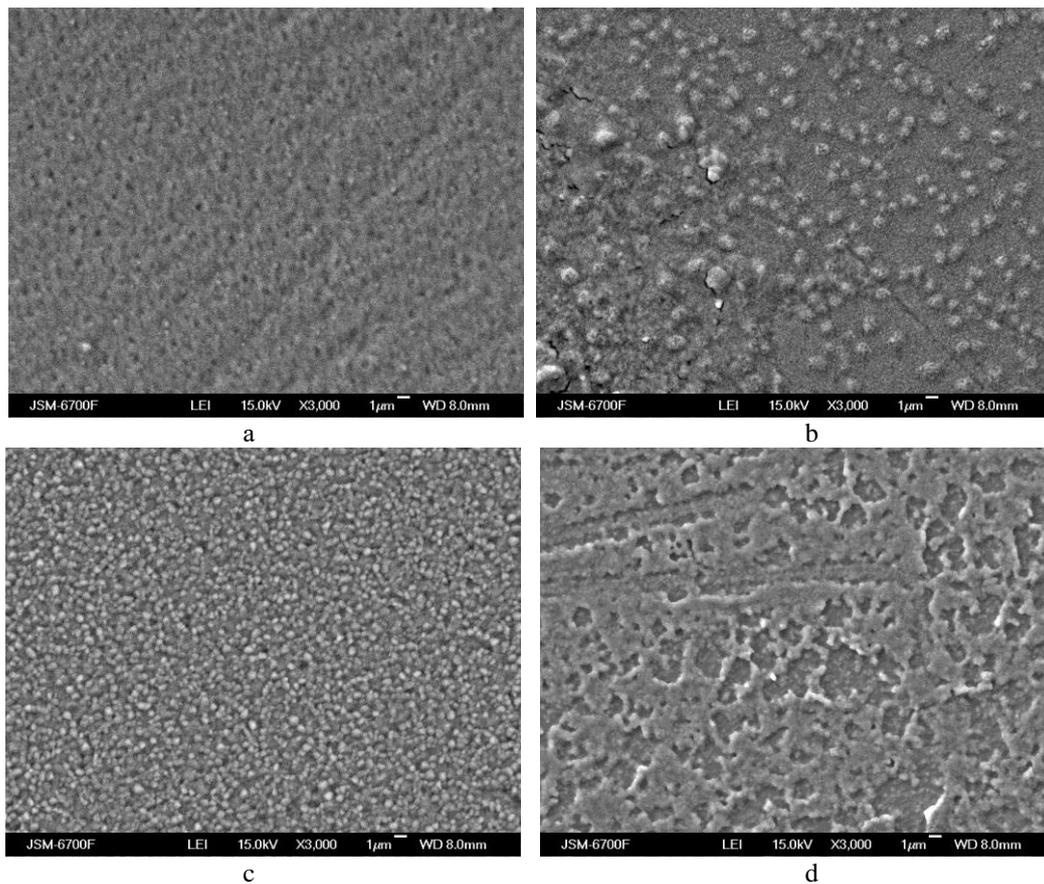
**Fig. 7.** SEM images of the zirconium nanofilms onto the ZrO<sub>2</sub>-ceramic after annealing in vacuum at 1600°C with different holding time: a – 2 min; b – 5 min; c – 10 min; d – 20 min.
