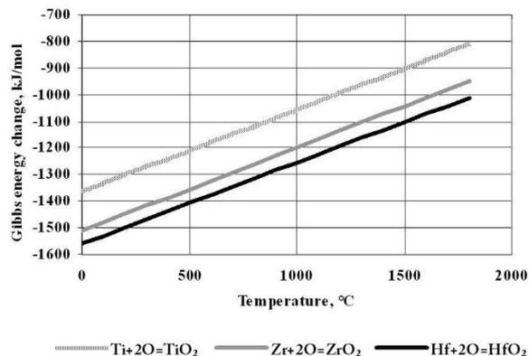
**Fig. 13.** Gibbs energy change for reactions of titanium, zirconium and hafnium to oxygen.
