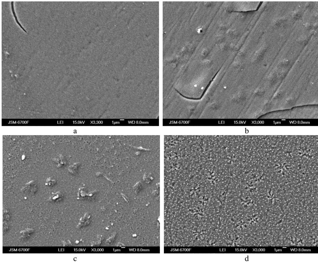
**Fig. 5.** SEM image of the zirconium nanofilms on the  $ZrO_2$ -ceramic after annealing in vacuum at  $1400^\circ C$  with different holding time: a – 2 min; b – 5 min; c – 10 min; d – 20 min.
